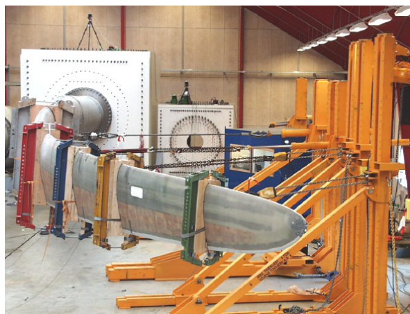
Figure 5: Structural test of a full wind turbine blade.
